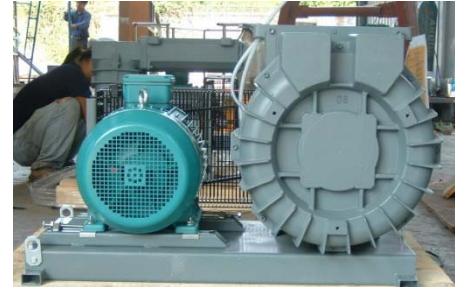
Central Vacuum Dust Collecting
