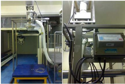
Bulk Bag Loading Station for Coffee-mate with metal detector
