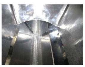
Inner part hard chromed coating to withstand the sand dust from sand paper
