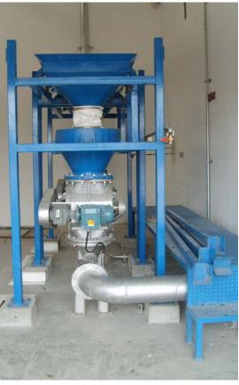
Bulk Bag Unloading Station for Bentonite clay powder
