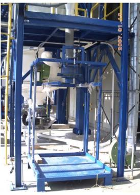
Bulk Bag Loading Station for paper pulp chip (raw material for dynamite bomb)
