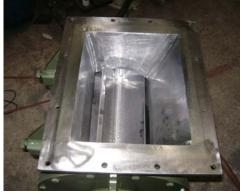
SIZE 14.0" ,carbon steel, for wood dust, pneumatic conveying system, plywood factory
